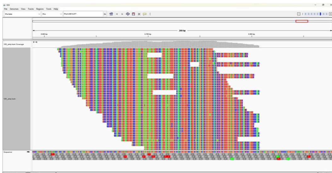
Figure 3. 24. Matching of the sequences obtained from the PCR screening of plant sample number 428 with the ampR partial primer to the pExpPN-phaA-SB vector using the Integrative Genomics Viewer program
