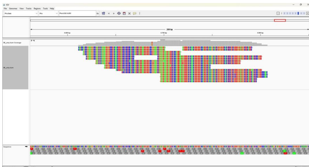
Figure 3. 22. Matching of the sequences obtained from the PCR screening of plant sample number 341 with the ampR partial primer to the pExpPN-phaA-SB vector using the Integrative Genomics Viewer program
