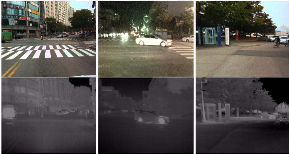
(b) Sample images from KAIST [96] dataset. Each column shows the visible and infrared image pairs exist in the dataset.
