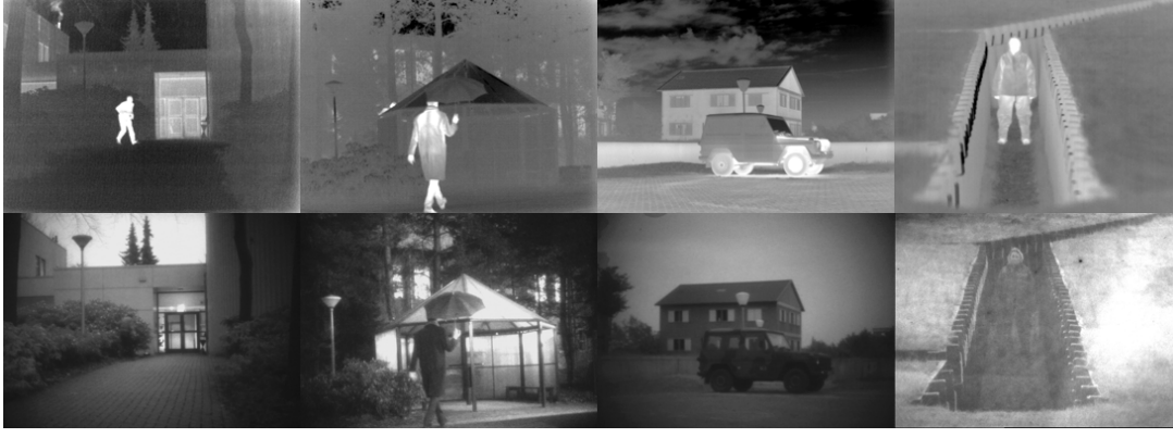
(a) Visible and infrared image pairs in TNO Dataset [2]. The sequence numbers are 12, 13, 16 and 21 from left to right respectively. Top row is infrared images while bottom row is visible images.
