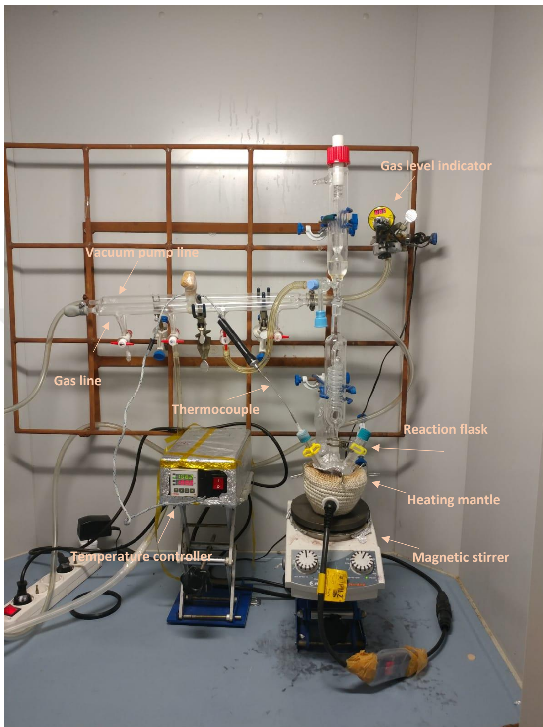
Figure 2.2: The Schlenk line apparatus and utilities employed for the synthesis under non-ambient conditions at our laboratory.
