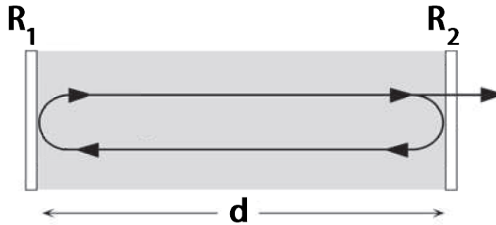
Figure 2.5: A Fabry-Pérot cavity of length d , a totally reflective mirror with a reflectance value R_1 , and a partially reflective mirror with a reflectance value R_2 .
