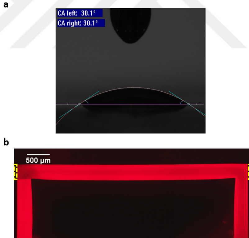
Figure 4.4: (a) Contact angle of toluene on treated PDMS, (b) fluorescent microscope image of capillary filled channel (shown with mirrors marked on the photograph).
