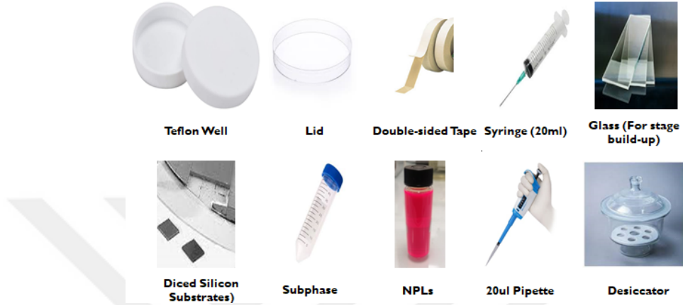
Figure 4.2: Instruments, tools, and materials used to carry out liquid-interface self-assembly.
