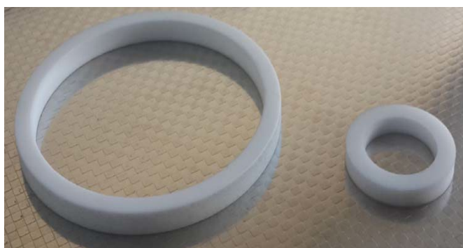
Figure 3.2. Deformable Teflon dies used in pressing.
