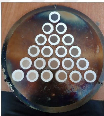
Figure 4.288. Symmetrical cells in a substrate holder after cathode coating.
