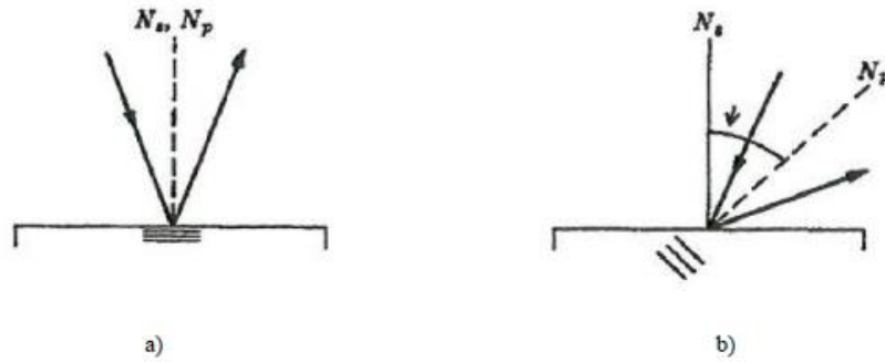
Figure 5.4 : Schematic illustration of measuring d_n at (a) and d_{\phi\psi} at (b) by diffraction, N_s is normal to specimen surface and N_p is normal to reflecting plane [84].
