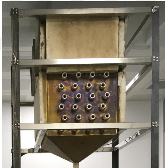
Figure 6.5. Hopper, with insulation removed to expose ends of the heating tubes.
