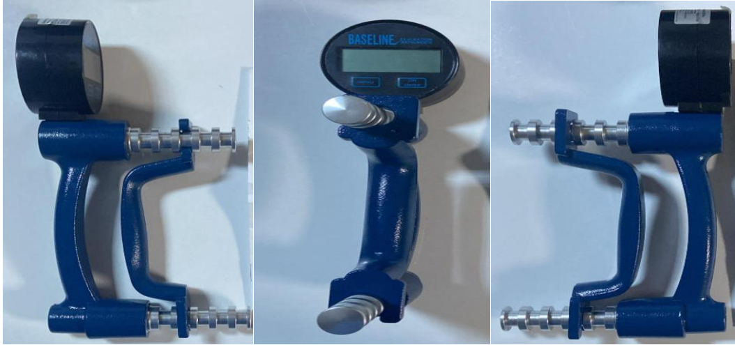
Şekil 33. El dinamometre cihazı, Baseline R instruction manual hydraulic hand dynamometer with digital LCD gauge
