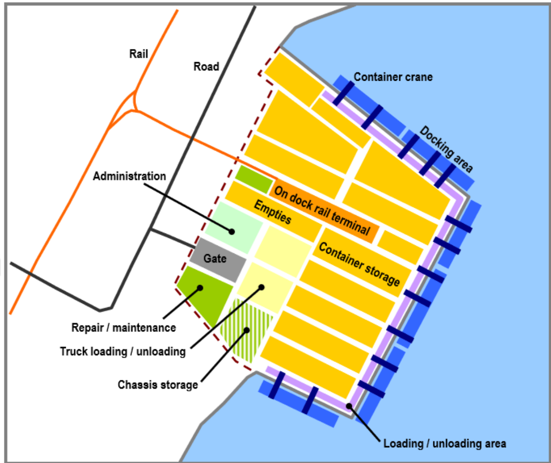
Figure 13: Configuration of a Container Terminal
