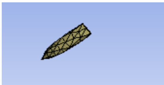
Figure 3.3 Meshed visual of 7.62 mm projectile
