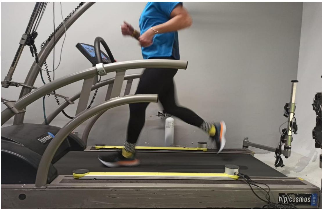
Figure 25: Running analysis with optojump system on H/P Cosmos Treadmill
