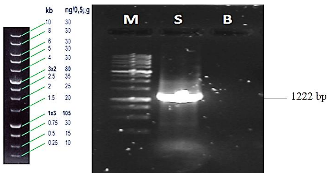
Figure 3.11 : PCR amplification of TpBGL2 from pPIC9 + TpBGL2 using ALFA and BGL2R primers (M: Marker (SHARPMASSTM 1 - DNA LADDER), B: Blank, S: Sample).
