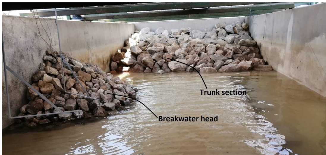
Figure 4.9 Locations of the breakwater head and trunk section in the channel
