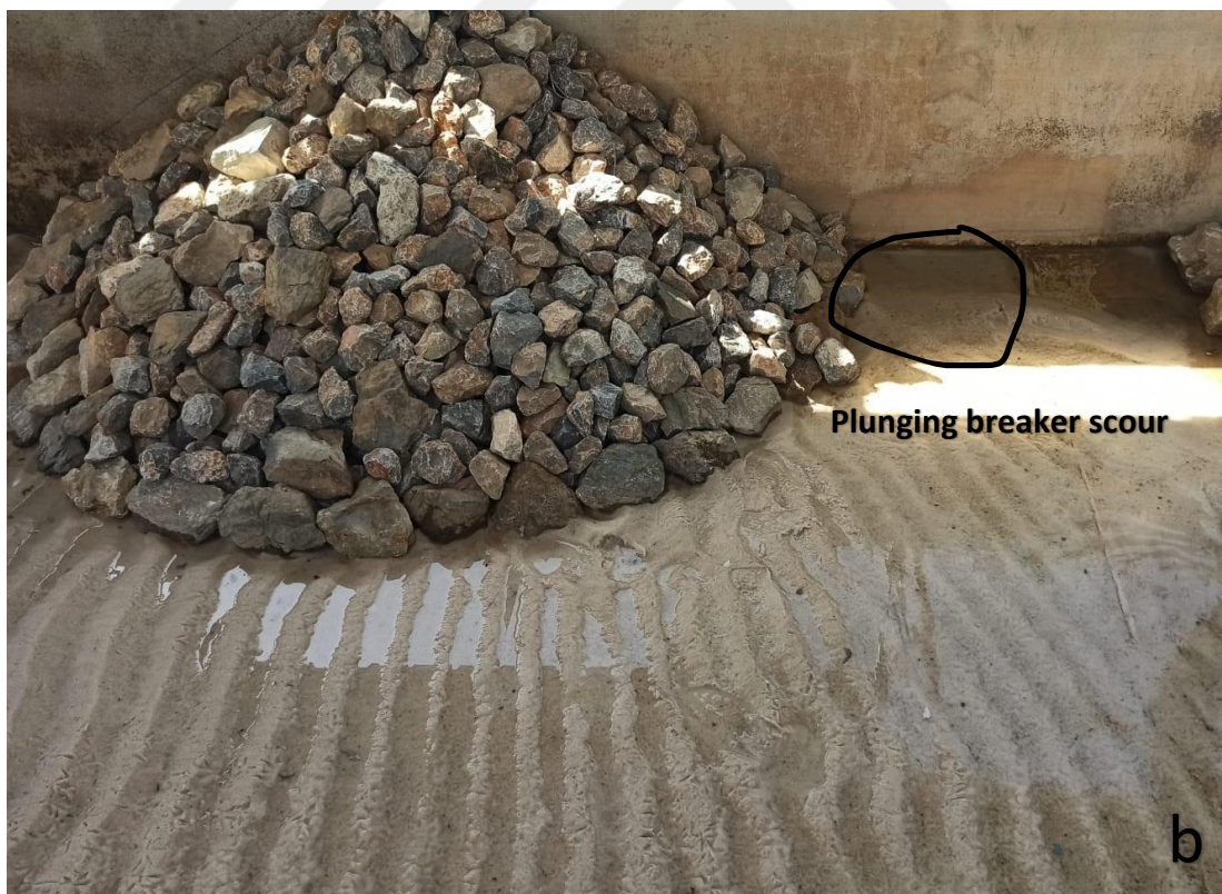
Figure 5.25 Bed topography (a) Breaking wave case, (b) Non-breaking wave case, Experiment No. B-1 and N-1
