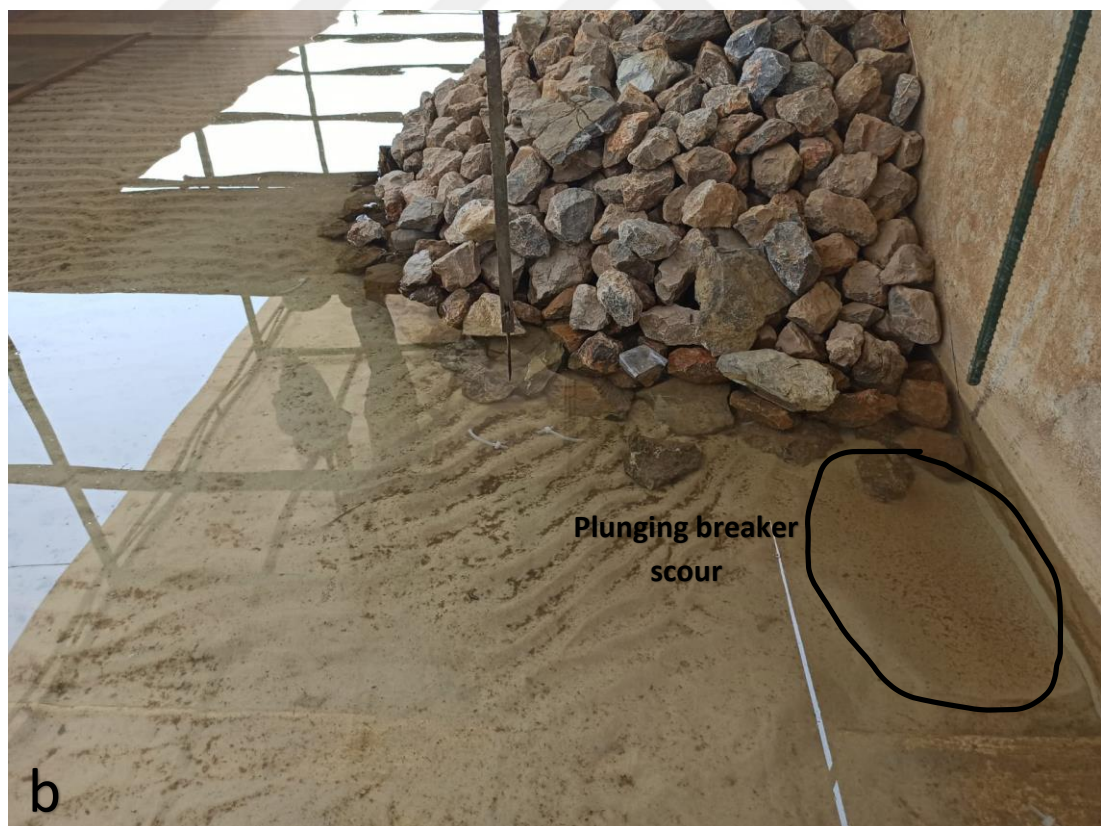
Figure 5.26 Bed topography (a) Breaking wave case, (b) Non-breaking wave case, Experiment No. B-5 and N-5
