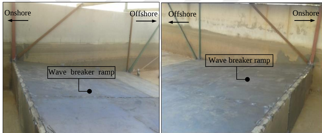
Figure 4.10 Two different views of the wave breaker ramp located in the channel
