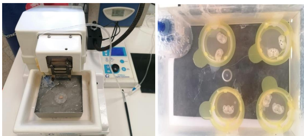
Fig11. (Left) Obtaining coronal brain slices in vibratome and (Right) obtained 250 \mu m-thick slices.
