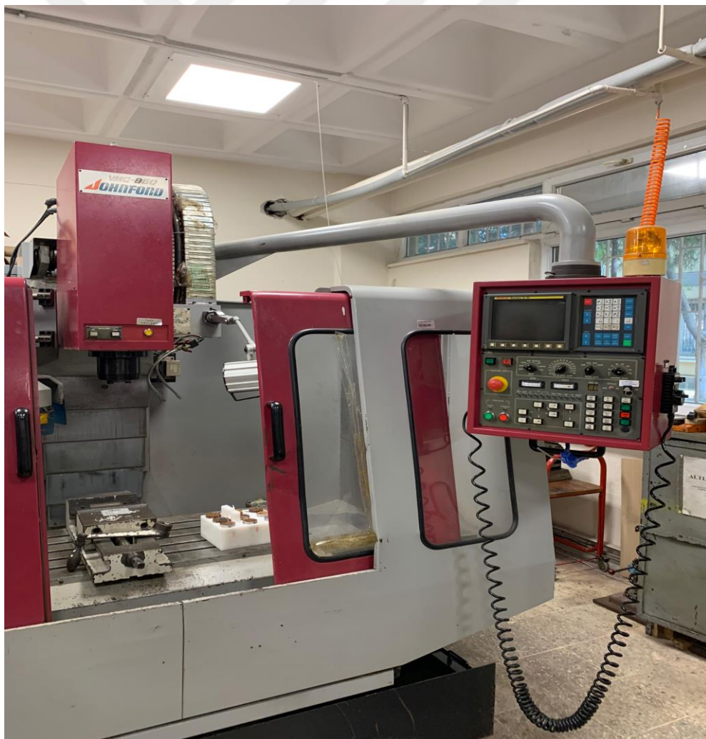
Figure 3.2. Johnford VMC-850 model CNC Milling machine (Taichung City, Taiwan)
