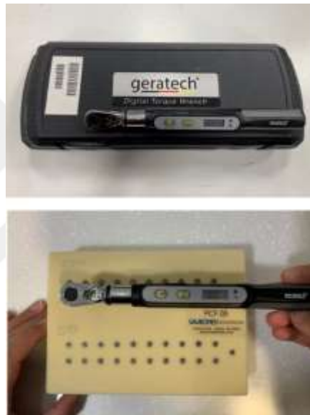
Figure 3.8. Geratech Digital Torque Wrench torque tool (Germany)
