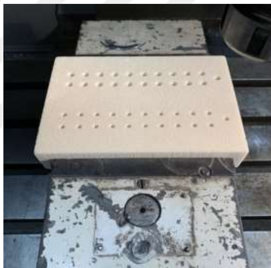
Figure 3.5. Implant slots opened to PCF05 and PCF020 bone type
