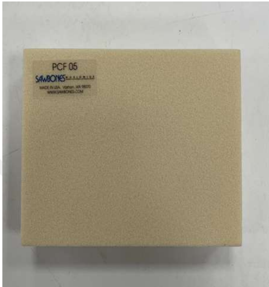
Figure 3.2. Sawbones, PCF05(D4) polyurethane bone (#1522-03: Malmo, Sweden)
