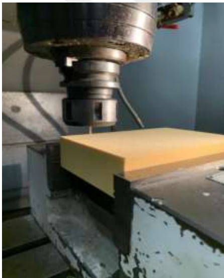
Figure 3.5. Implant slots opened to PCF05 and PCF020 bone type
