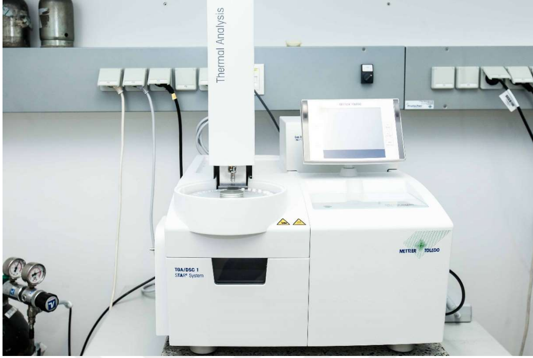
Şekil 11. “Mettler Toledo DSC 1 Star System” DSC (Differential Scanning Calorimetry) Cihazı
