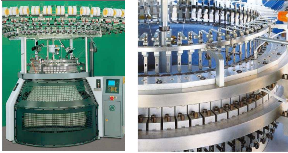
Şekil 2.5 “Single-jersey” yuvarlak örme makinesi (Mayer, (b.t.) ve Terrot, (b.t.)).
