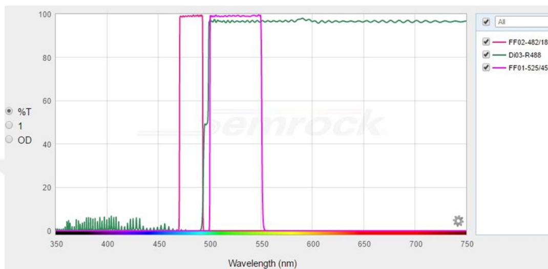
Figure G 1 Excitation and emission ranges of EGFP filter used in Leica DMI4000 B with Andor DSD2 Confocal device.
