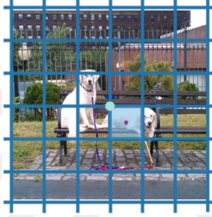
Figure 2.5: A sample figure to represent the idea of the grid cells. Purple point in the center of the cell is the center point (X, Y) of the bounding box to be proposed and the green point (x, y) is the coordinate of the grid cells' itself. The image taken from COCO dataset [2]
