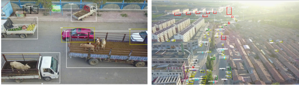
Figure 3.4: Two sample images demonstrate how the viewing angle and the object scales change an object’s appearance in an UAV-taken image. Both of the sample images are taken from the VisDrone2019 [4] dataset.
