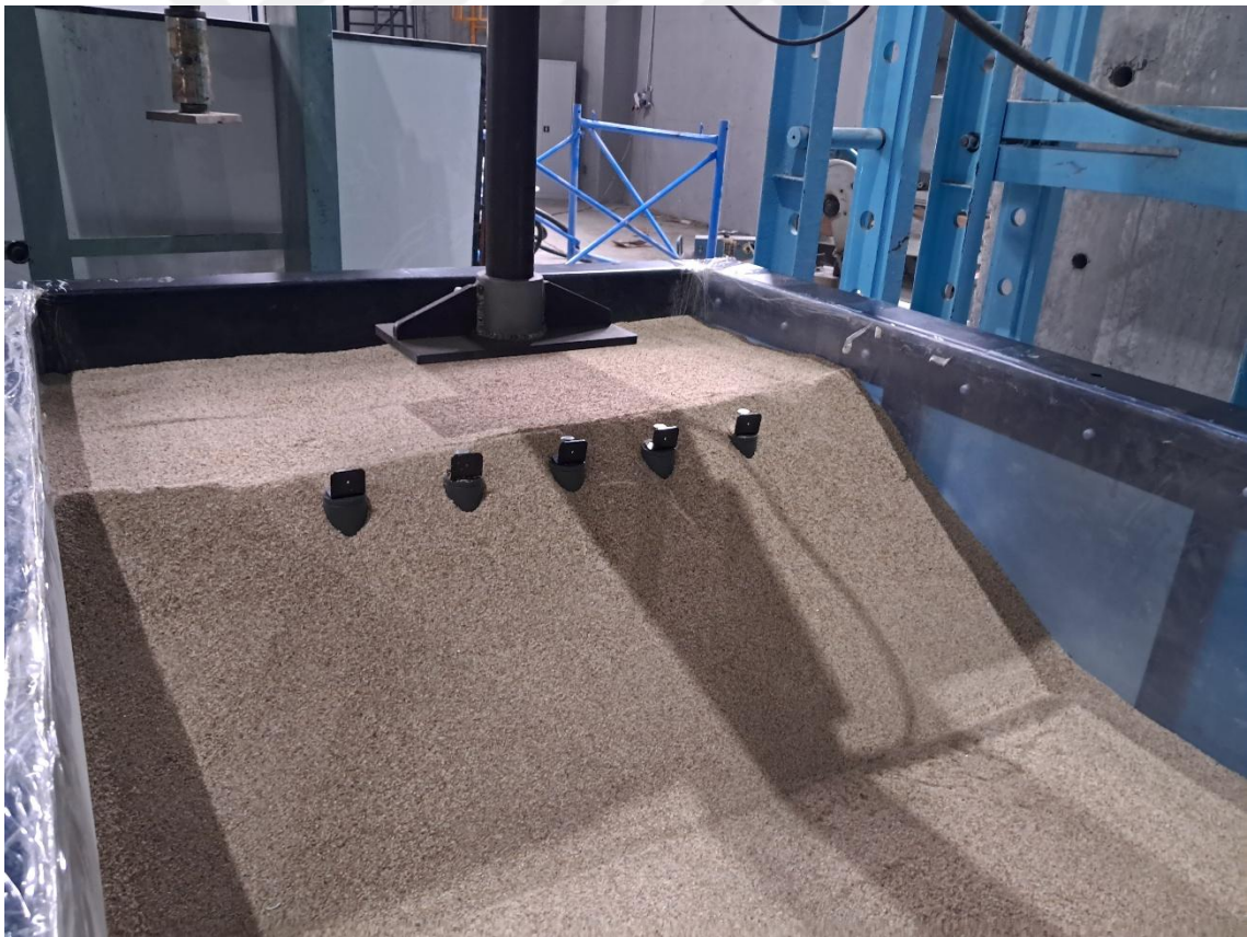
Figure 3.20. Experimental test setup with piles.
