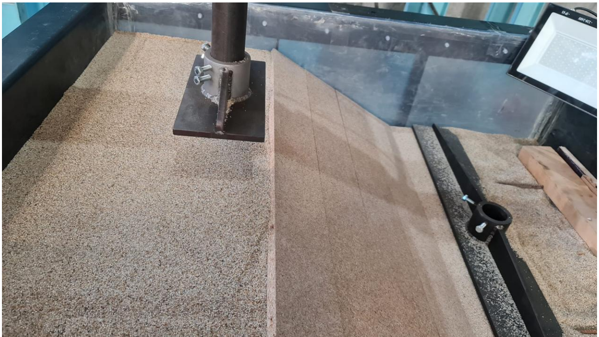
Figure 3.3. Picture depicting assembled mold after soil placement.
