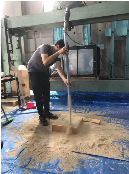
Figure 3.13. A photo depicting sand placement into the wooden calibration box using pluvation technique.
