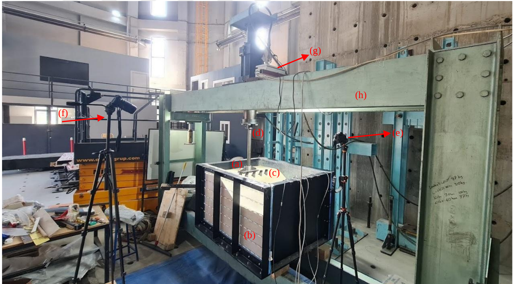
Figure 3.21. Experimental Setup (a) local loading plate, (b) model tank, (c) piles, (d) hydraulic jack, (e) camera 1, (f) camera 2, (g) control box, (h) loading frame.
