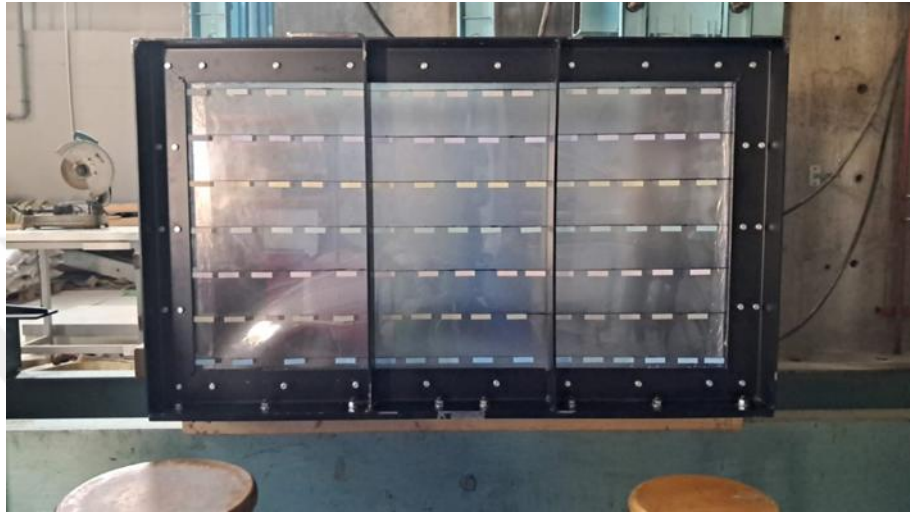
Figure 3.16. The plexiglass side-view of the physical model test tank with layer markings.
