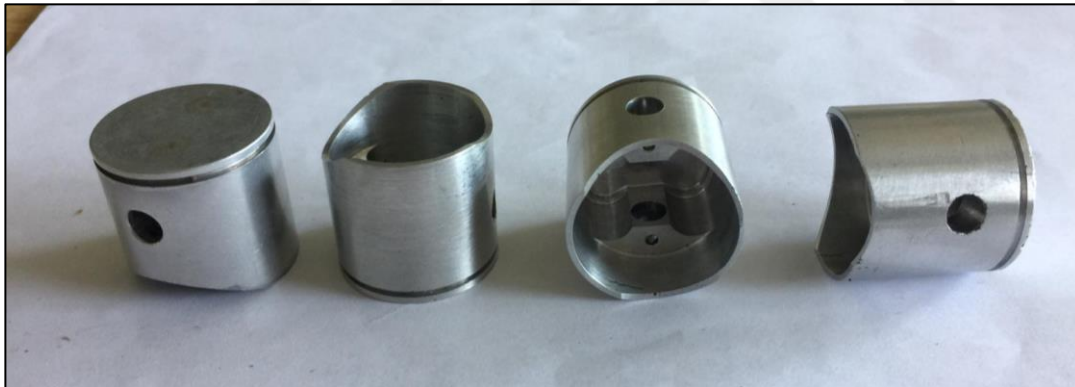
Figure 3.25. Pistons after squeeze casting and machining.
