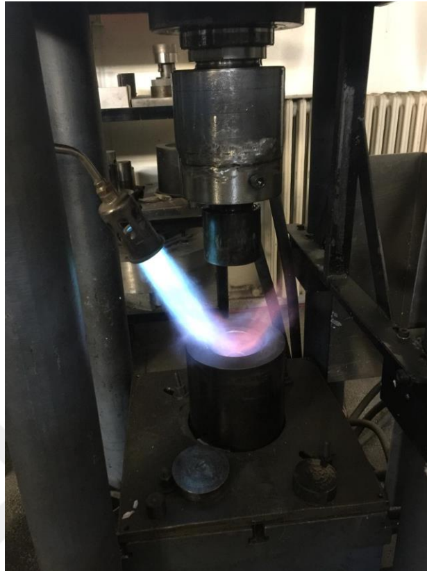
Figure 3.19. Heating the mold to 100 °C.
