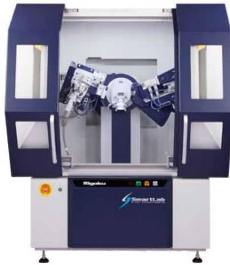
Figure 3.28. A typical XRD machine [49].
