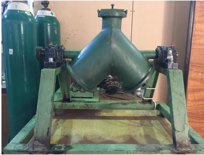
Figure 3.18. V type mixing machine used for Al based and SiC powders.
