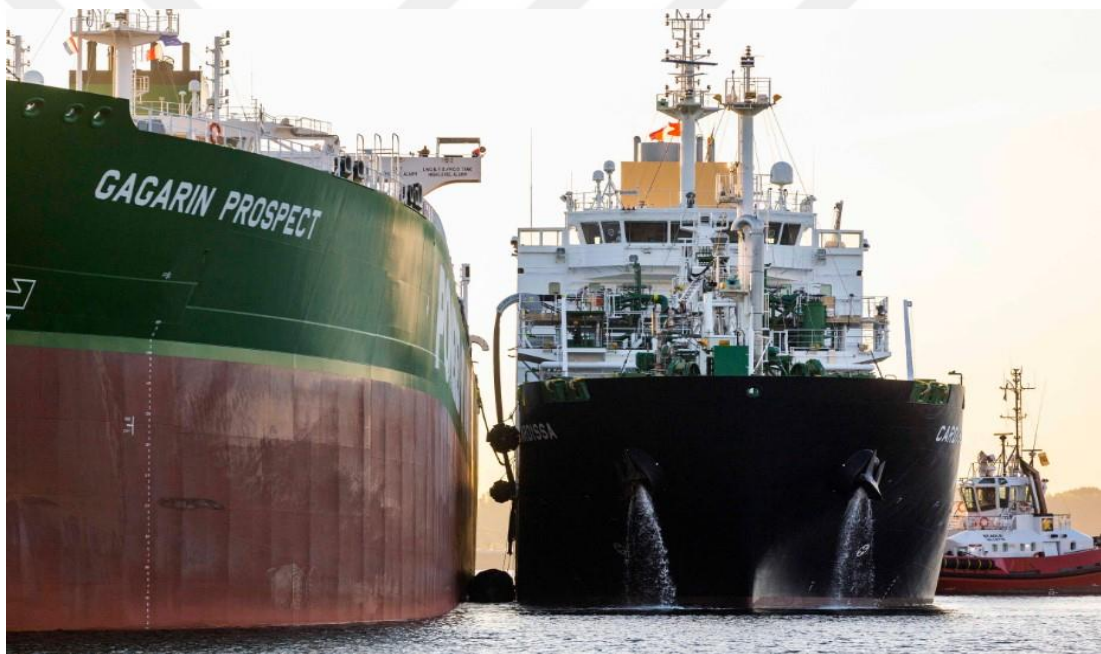
Figure 46: Ship to Ship Bunkering Operation
