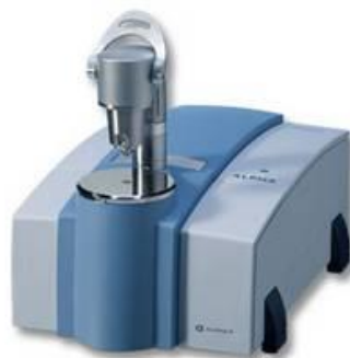
Figure 4.6 Bruker ALPHA Platinum ATR single reflection diamond based ATR spectrometer that was used in this study. Taken from ref #72.
