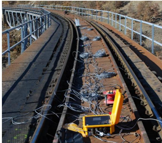
Figure 3.14 Data acquisition device (Personal archive, 2015)
