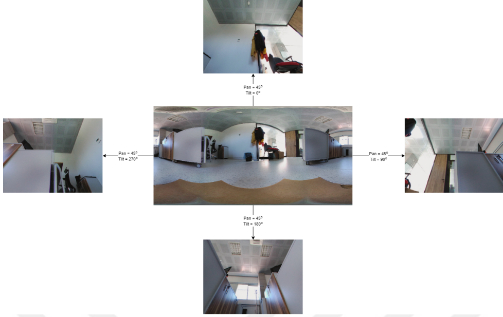
Figure 2.1: Rectification at 0^\circ (top), 90^\circ (right), 180^\circ (bottom), 270^\circ (left) Pan Angles
