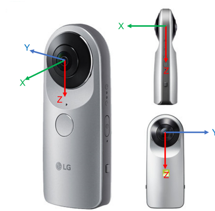
Figure 3.7: Panoramic camera used in capturing images and axes used
