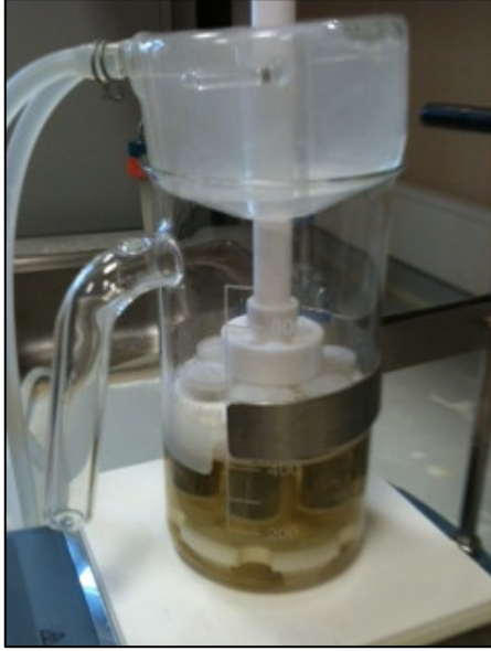
Figure 3.3. A picture of Lignin analysis content of litterfall. Capsule tray with 6 positions in extraction beaker with a condenser was on the hot plate.
