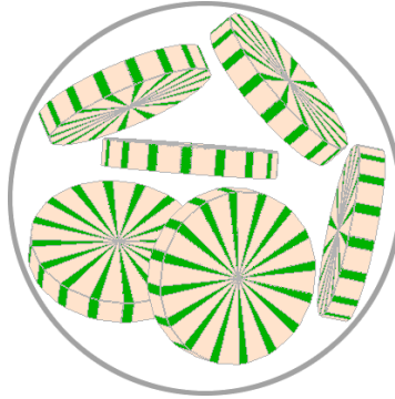
Figure 5.1: Randomly oriented realizations of the disk-like spherulite model. Dark and light regions are amorphous and crystalline, respectively.
