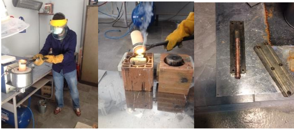
Figure 2.12 Images captured while producing samples during the casting process
