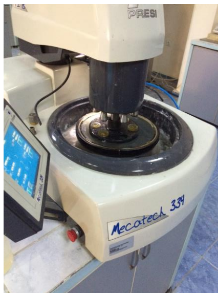
Figure 2.13 Mecatech 334 Automatic Grinding Machine using for metallographic studies
