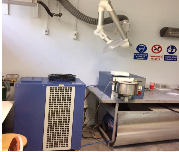
Figure 2.8 Induction furnace system used in the casting process
