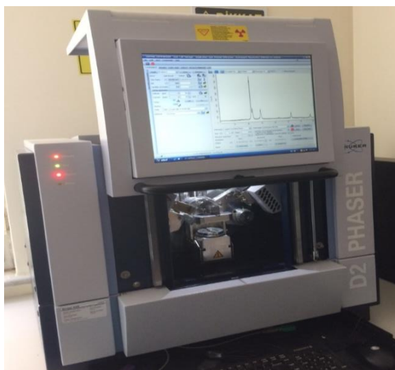
Figure 2.10 X-ray diffraction instrument for phase detection
