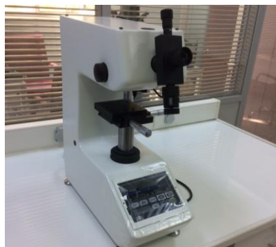
Figure 2.18 HMV-2T Shimadzu brand hardness tester used for determination of microhardness.
