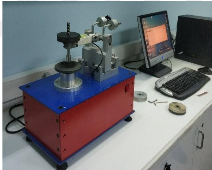
Figure 2.19 Pin-on Disk Tribometer Device used for determination of wear rate
