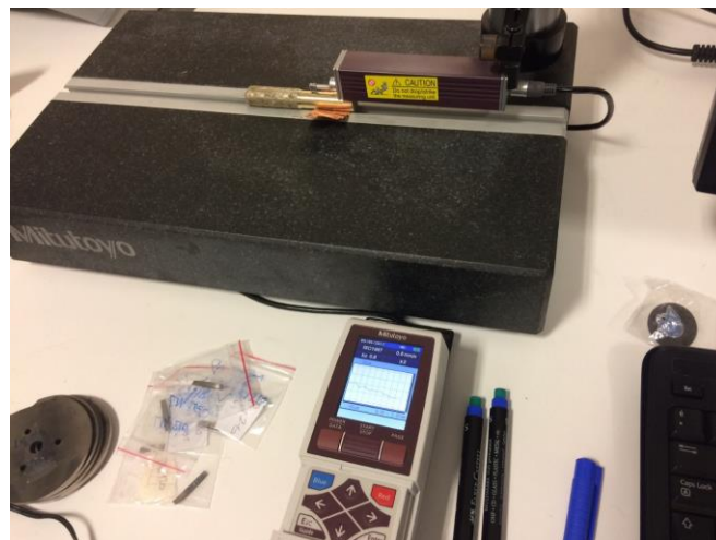
Figure 2.16 Surface Roughness Testers MITUTOYO SJ-201P
