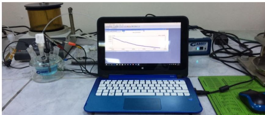
Figure 2.15 Standard electrochemical cell used for determination of corrosion rate
