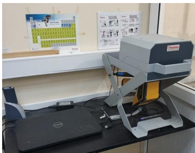
Figure 2.11 The Portable XRF Spectrometry for determination of chemical composition
