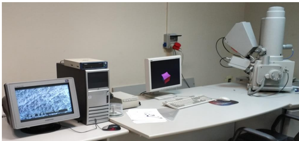
Figure 2.9 Scanning Electron Microscope for microstructure analysis
