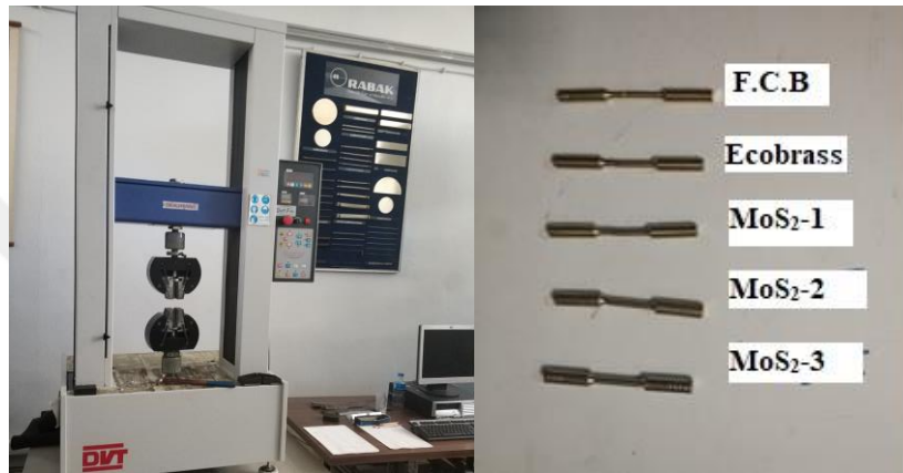
Figure 2.17 The images of tensile testing instrument and tested samples
