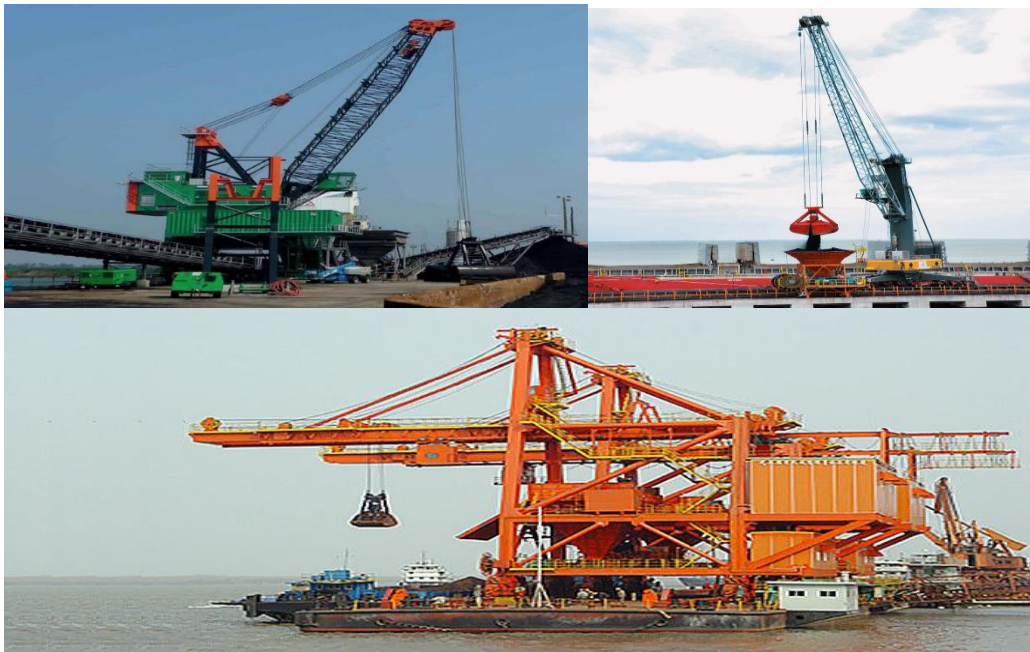
Figure 10: Dry Bulk Grab Unloading Equipment
