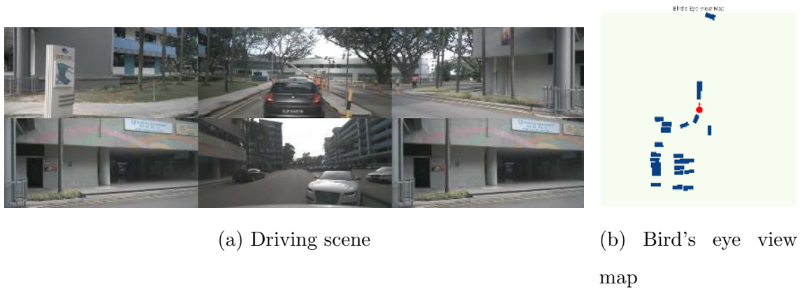
Figure 1.1: An example of camera images from a driving scene in nuScenes paired with its Bird's Eye View (BEV) representation. The ego vehicle is denoted by a red circle at the center of the BEV, with its front facing upward. Other vehicles are represented in blue.
