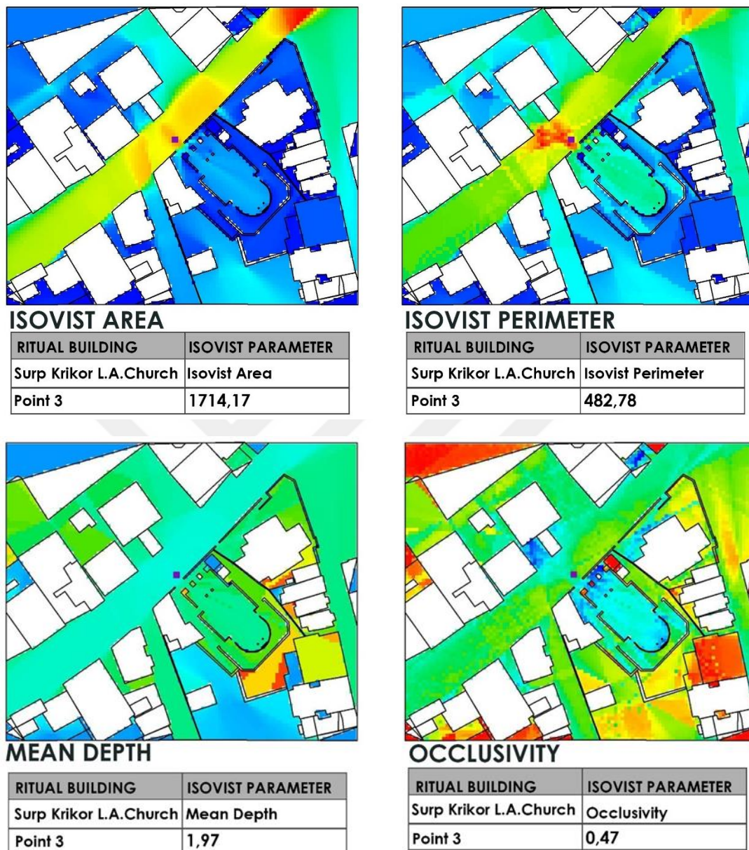
Figure 97: Isovist Area, Isovist Perimeter, Mean Depth, Occlusivity values (Point 3) of Surp Krikor Lusavoric Armenian Church
