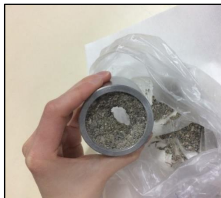
Figure 3.33. Removing specimen from the mold
