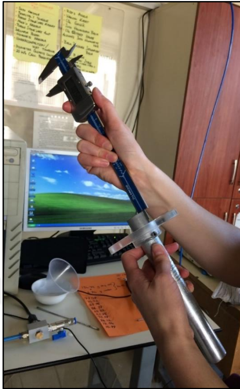
Figure 3.9. Height adjustment of the tamping rod
