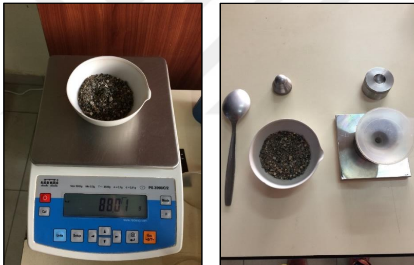
Figure 3.26. Pieces of equipment used for specimen preparation; a bowl, balance, spoon, funnel, oedometer mold and top cap
