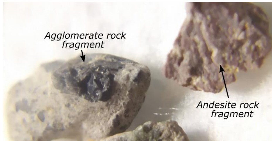
Figure 3.2. Agglomerate and andesite rock fragments ( 2 – 3 mm diameter) observed in Kızılırmak sand
