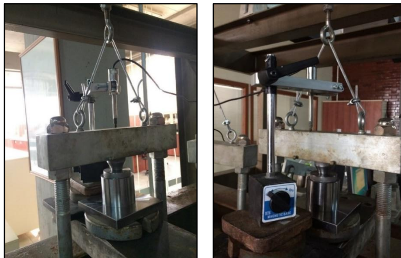
Figure 3.30. Placement of the LVDT on the loading frame
