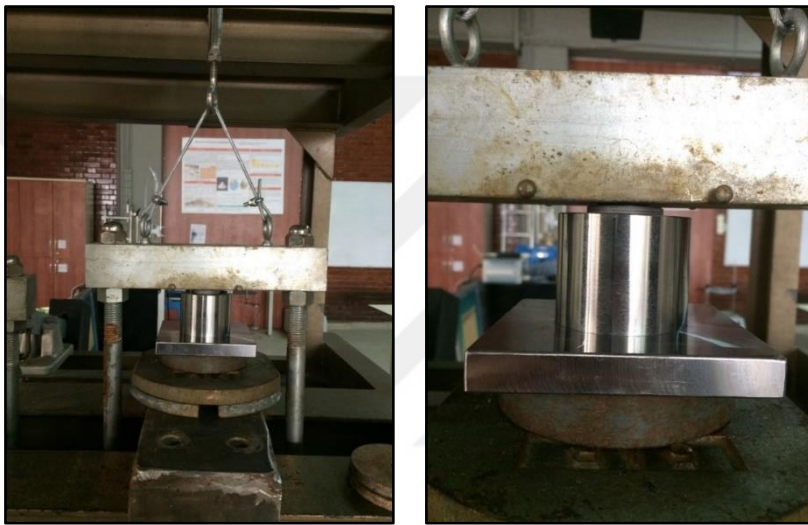
Figure 3.29. Placement of the prepared specimen under the loading frame
