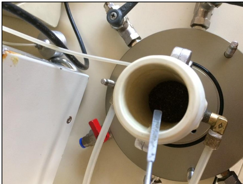
Figure 3.14. Scratching the compacted surface
