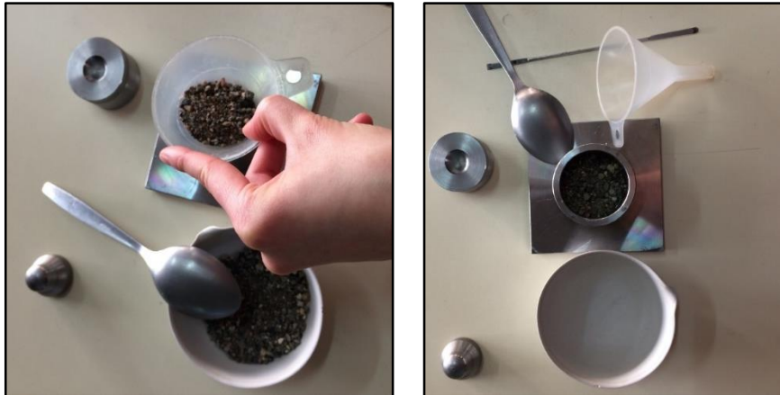
Figure 3.27. Dry pluviation process and the sample after the completion of pluviation
