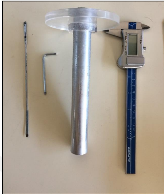
Figure 3.8. Tamping rod and caliper
