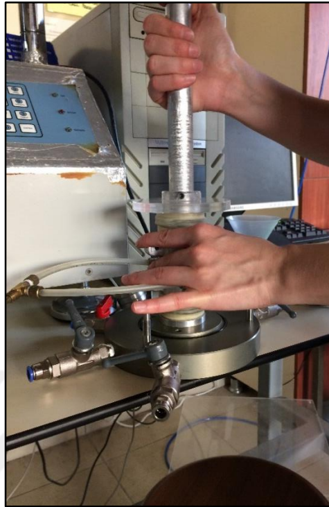
Figure 3.13. End of the compaction process
