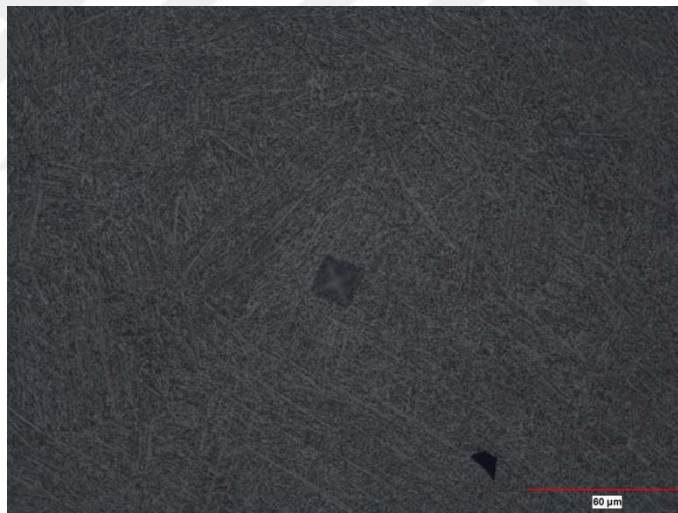
Figure 4.36. Example of vickers indentation image of anneal heat treated material
