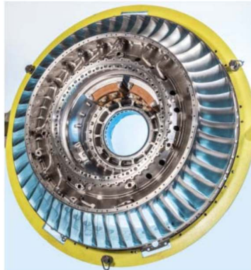
Figure 1.4. Titanium additive part application examples of Rolls Royce Trent XWB engine front bearing bed (Özsoy et al., n.d.)
