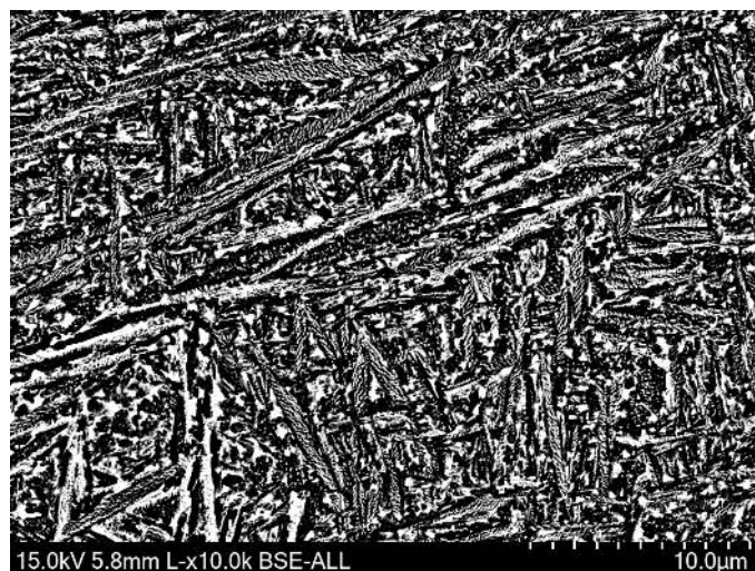
Figure 4.4. SEM microstructure at annealed condition
