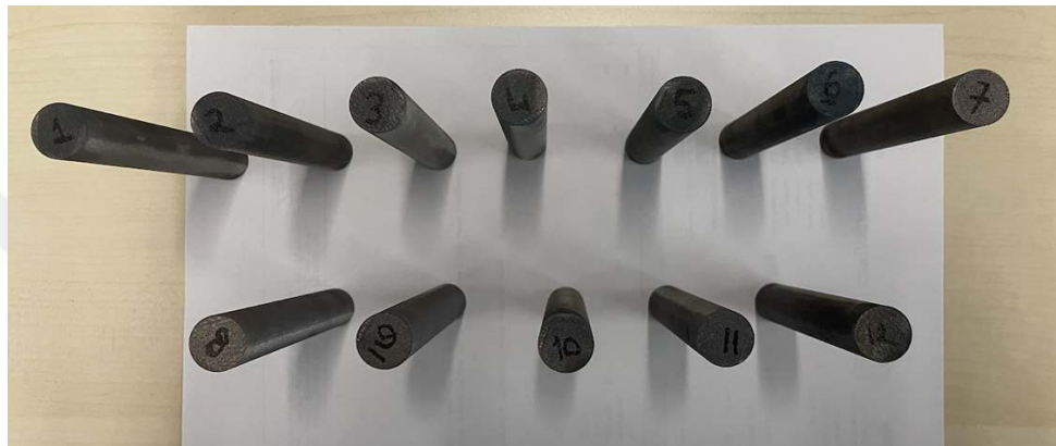
Figure 3.7. HIPed specimens after HIP process and before the machining
