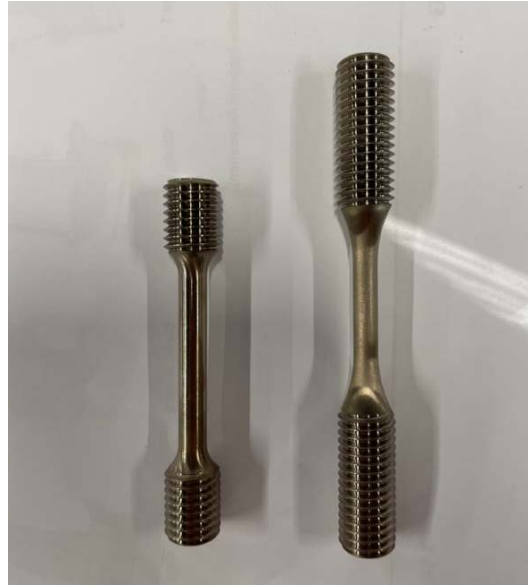
Figure 3.6. Machined specimens for fatigue and tensile tests
