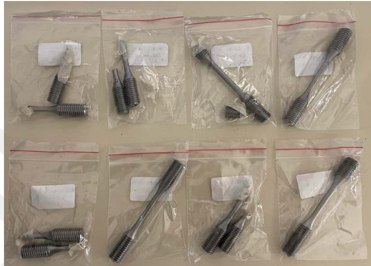
Figure 3.9. Some of fatigue coupons whose fracture surfaces were examined
