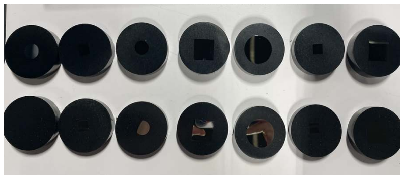
Figure 3.8. Microstructure coupons for optical microscope and SEM examinations
