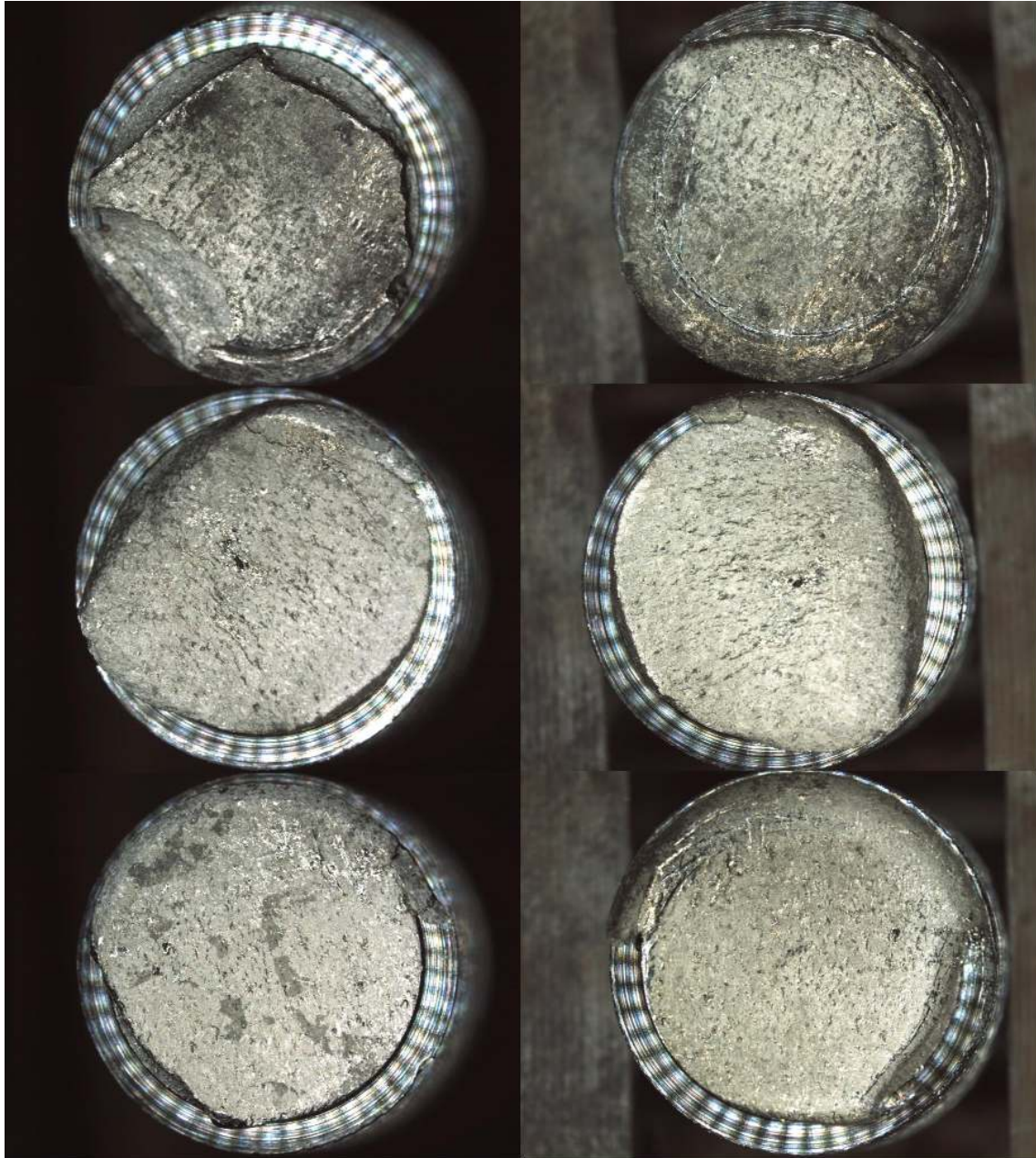
Figure 4.10. Z direction annealing heat treated fatigue specimens from radius and thread sections
