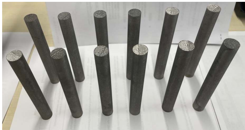
Figure 3.5. The some of fatigue test specimens produced for the thesis after SLM production.
