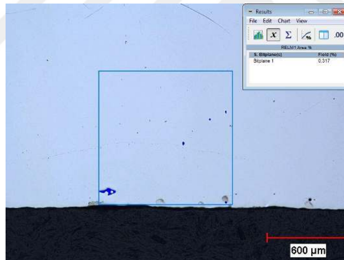
Figure 4.31. Before HIP sharp porosity in coupon 5
