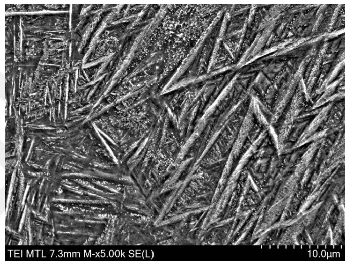
Figure 4.2. SEM microstructure at as-built condition
