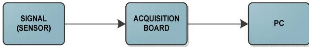
Figure 2.1 A typical structure of DAQ system [12]
