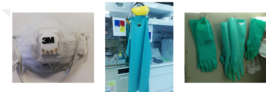
Figure A.3: Images of an N-95 mask; the gown and helmet; and the acid-resistant gloves used for personal protection during the etching process
