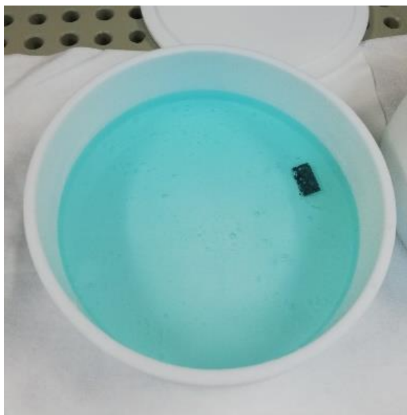
Figure A.6: Image of a sample placed inside the chemical etchant
