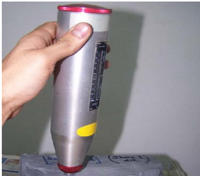
Figure 5.17: A Typical L-type Schmidt rebound hardness device.
