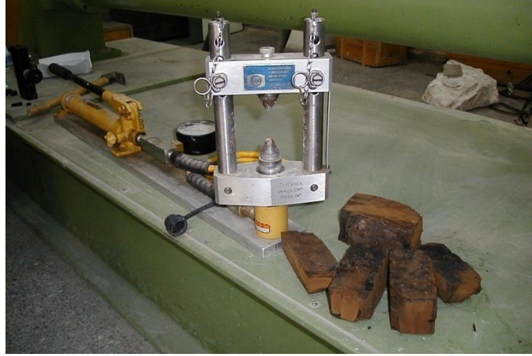
Figure 5.19: Point load test equipment.
