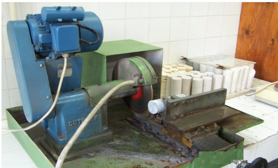
Figure 5.12: Typical core diamond sawing machine.
