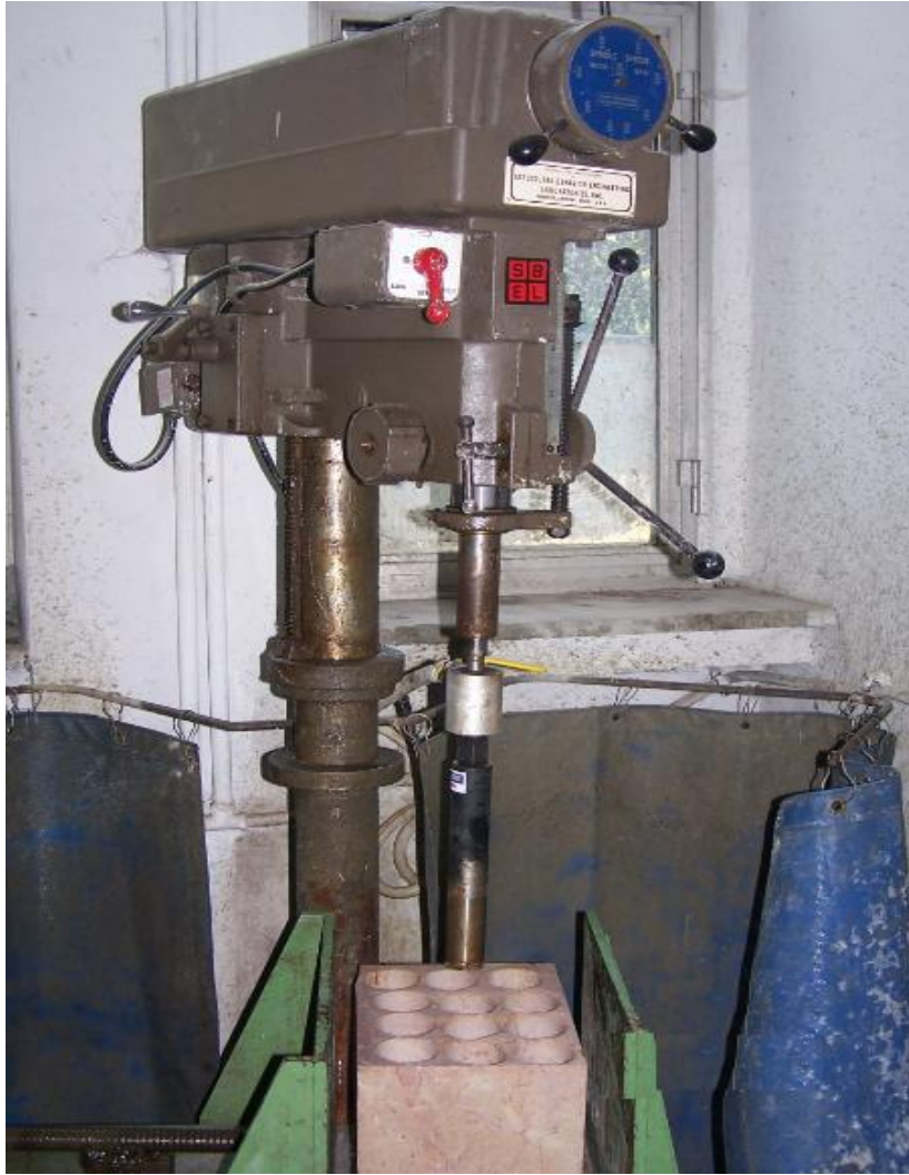
Figure 5.11: Typical core drilling machine.
