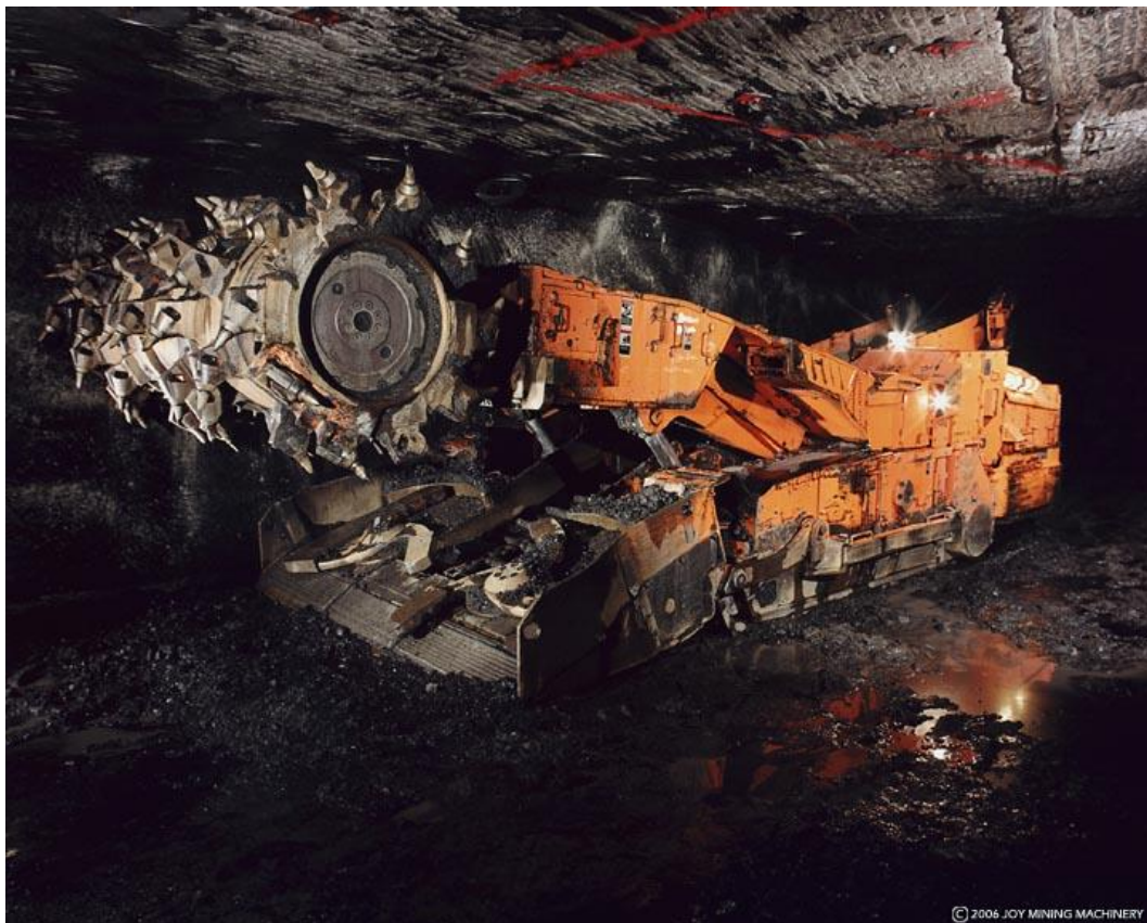
Figure 2.3: A typical continuous miner.
