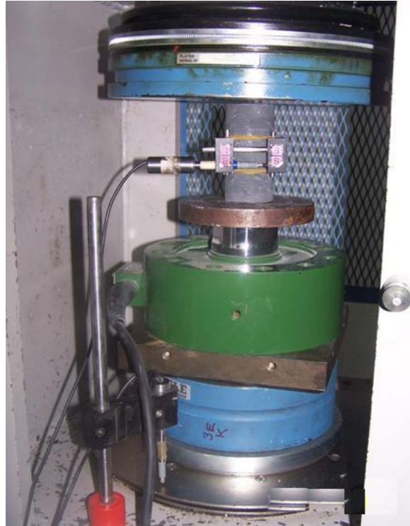
Figure 5.14: ELE- Autotest 3000 model UCS testing machine.
