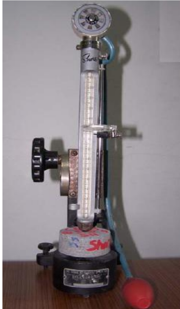
Figure 5.18: Typical Shore scleroscope hardness device.
