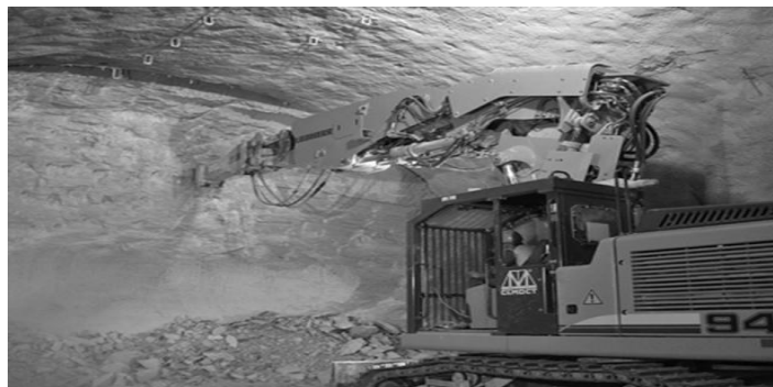
Figure 2.4: A typical impact hammer.
