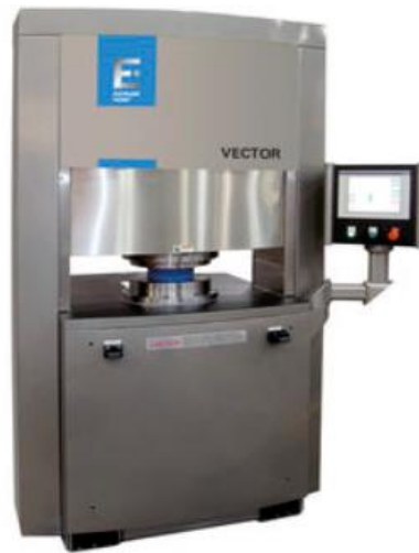
Figure 4.10 Extrude Hone Abrasive Flow Machine
