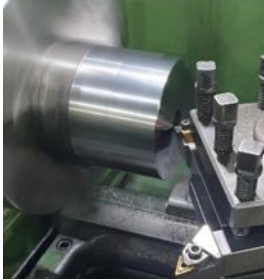
Figure 2.24 Front Diamond Protruding As A Result of Clamping
