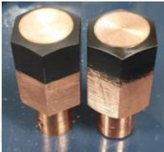
Figure 3.13 Copper Electrodes Formed Base Form
