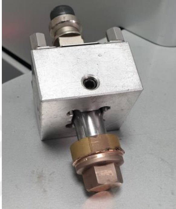
Figure 3.19 Radius Formed, Carbide Alloyed Copper Electrode
