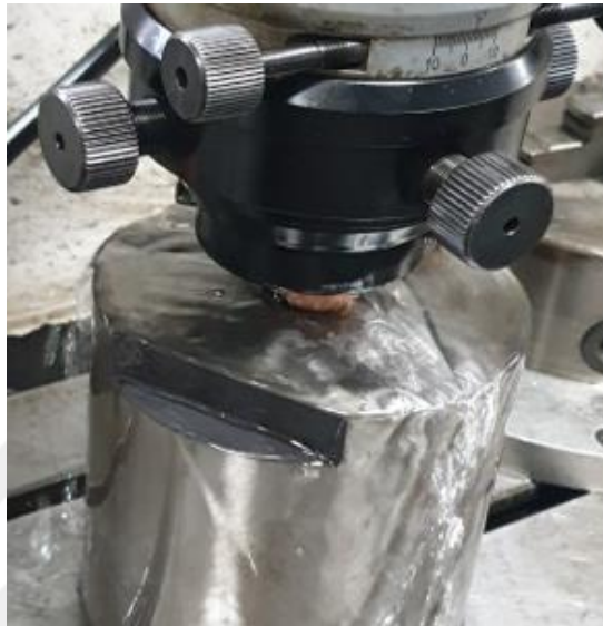
Figure 2.26 Base Form Machining Process in Sinker Erosion Machine
