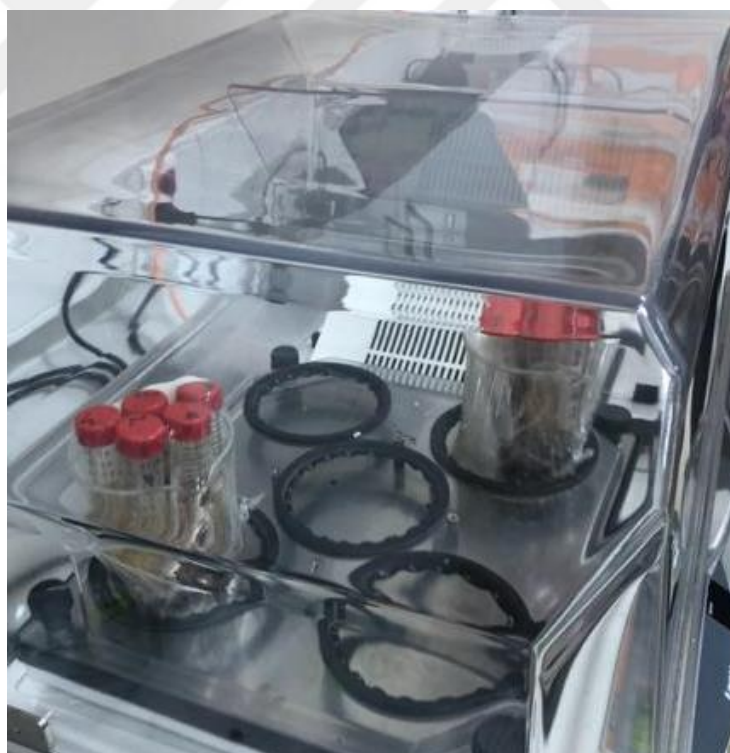
Figure 11. Operation picture of alkali pretreatment in shaking incubator. (samples are labeled and noted for different varying parameters: temperature, operation time and solvent ratio)
