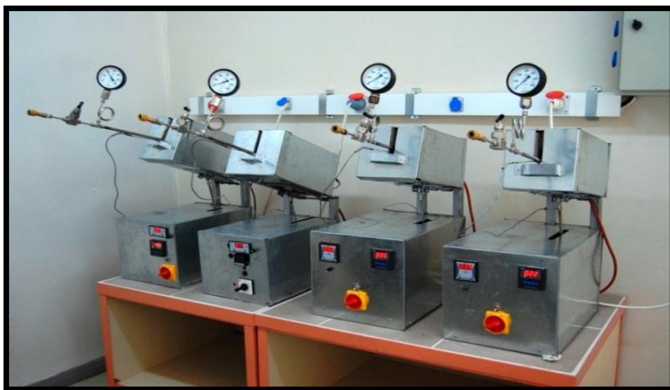
Figure 4.1.2 Heater and autoclave batch system.
