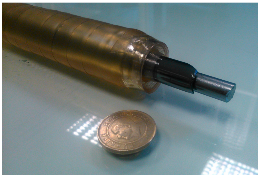
Figure 5.9: The preform was prepared for the first step drawing.
