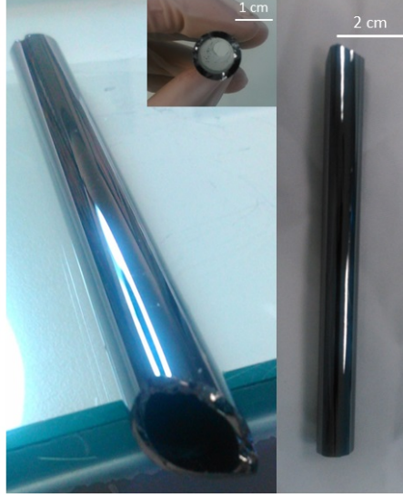
Figure 4.10: The Ge_{10}As_{23}Se_{67} tube fabricated by rotational casting
