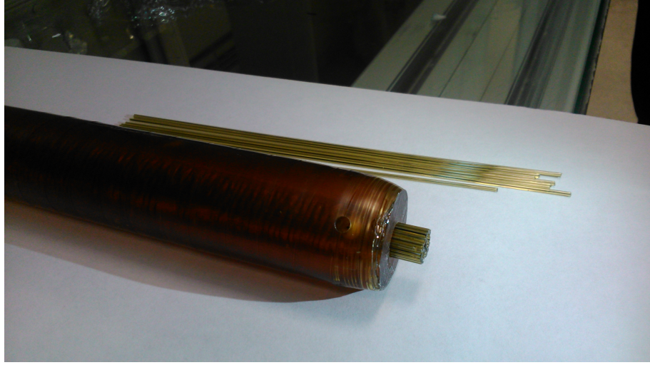
Figure 5.12: The preform was prepared for the third step fiber drawing. The second step fibers with seven-core structure were placed to another polymer tube to draw the third step fiber and to obtain the desired diameter.
