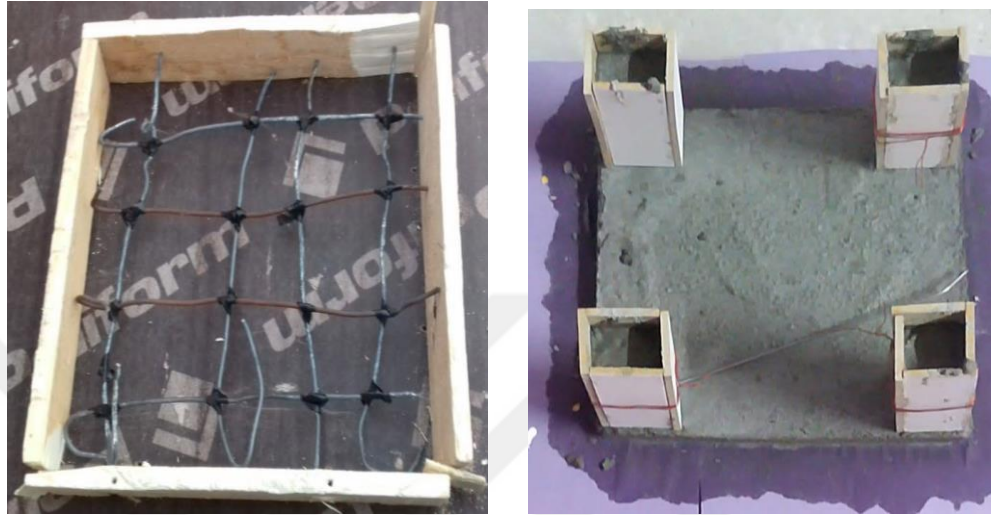
Figure 4.9. Some students' molds with cement mortar
