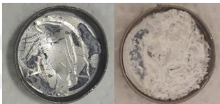
Figure 4.9 Metallic lithium anode under inert atmosphere (left) and degradation of metallic lithium anode after exposed to air (right).
