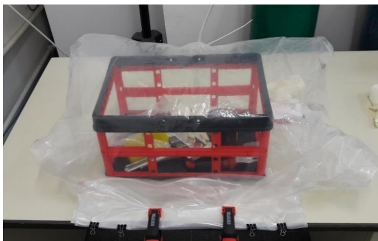
Figure 4.10 Photo of the setup where the batteries are disassembled: Glove bag filled with N_2 gas.
