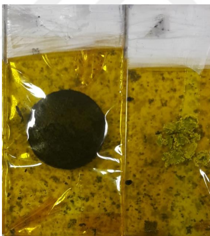
Figure 4.11 The cathode (left) and the anode (right) material of a non-rechargeable CR2032 coin cell battery fixed onto microscope slide and sealed with Kapton tape.
