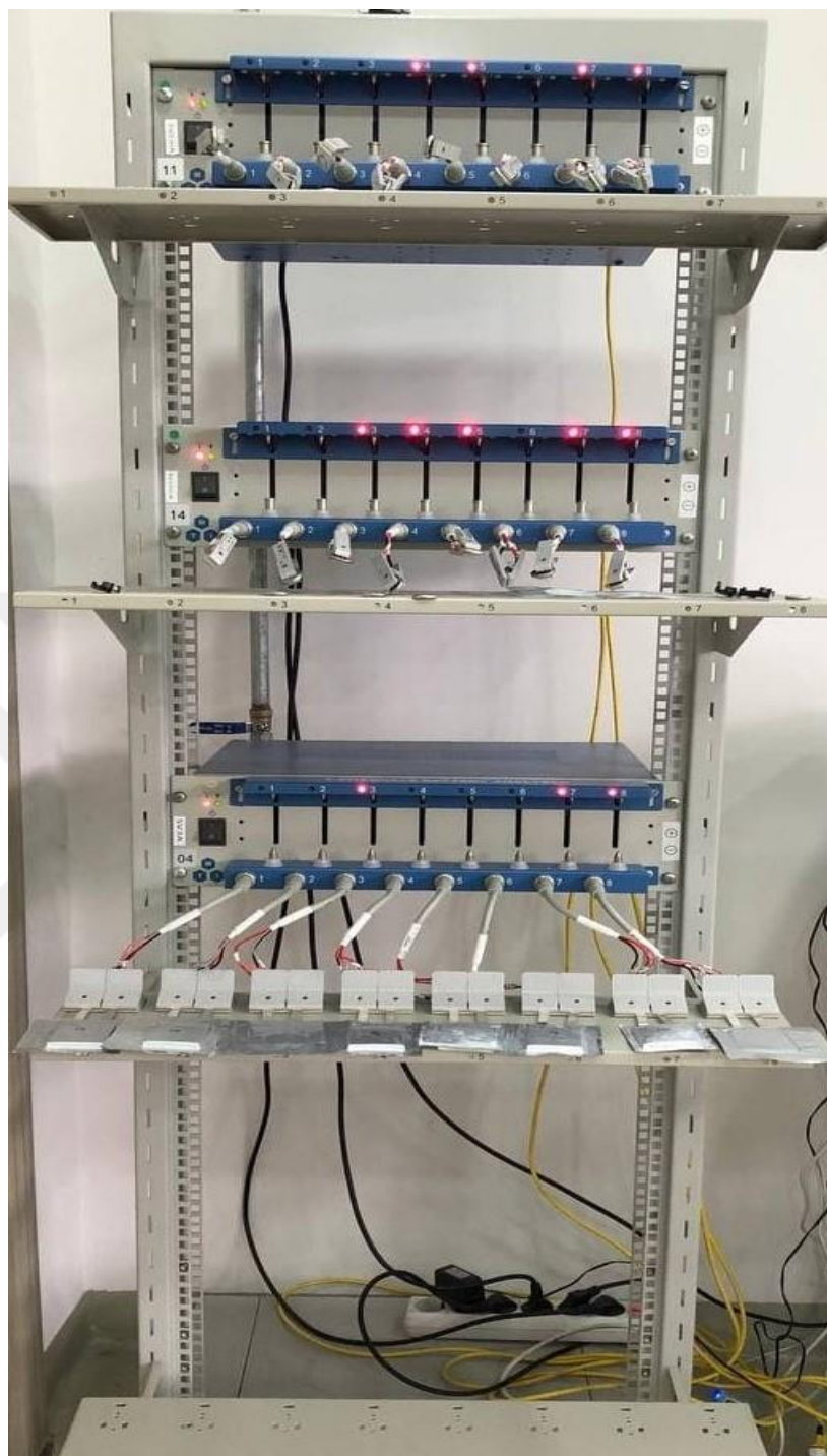
Figure 4.11. Coin cell battery test system.
