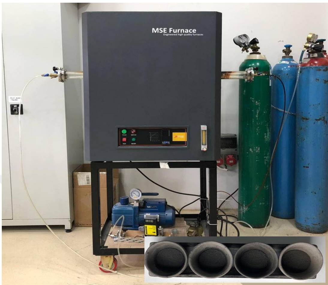
Figure 4.6. Tube furnace for sintering the dried precursor.
