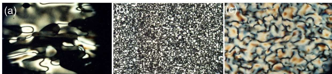
Figure 1.5. Characteristic magnetically non-well aligned textures of lyotropic nematic phases observed under polarising optical microscope: (a) N_D , (b) N_B and (c) N_C .
