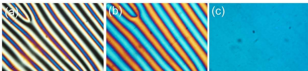
Figure 1.6. Magnetically well-aligned lyotropic cholesteric textures of (a) Ch_D , (b) Ch_B and (c) Ch_C phases. The Ch_C phase is unwound under the effect of external magnetic field, i.e. helical structure is destroyed and its texture is similar to well-aligned N_C phase. The distance between three parallel lines in (a) and (b) corresponds to the pitch length.
