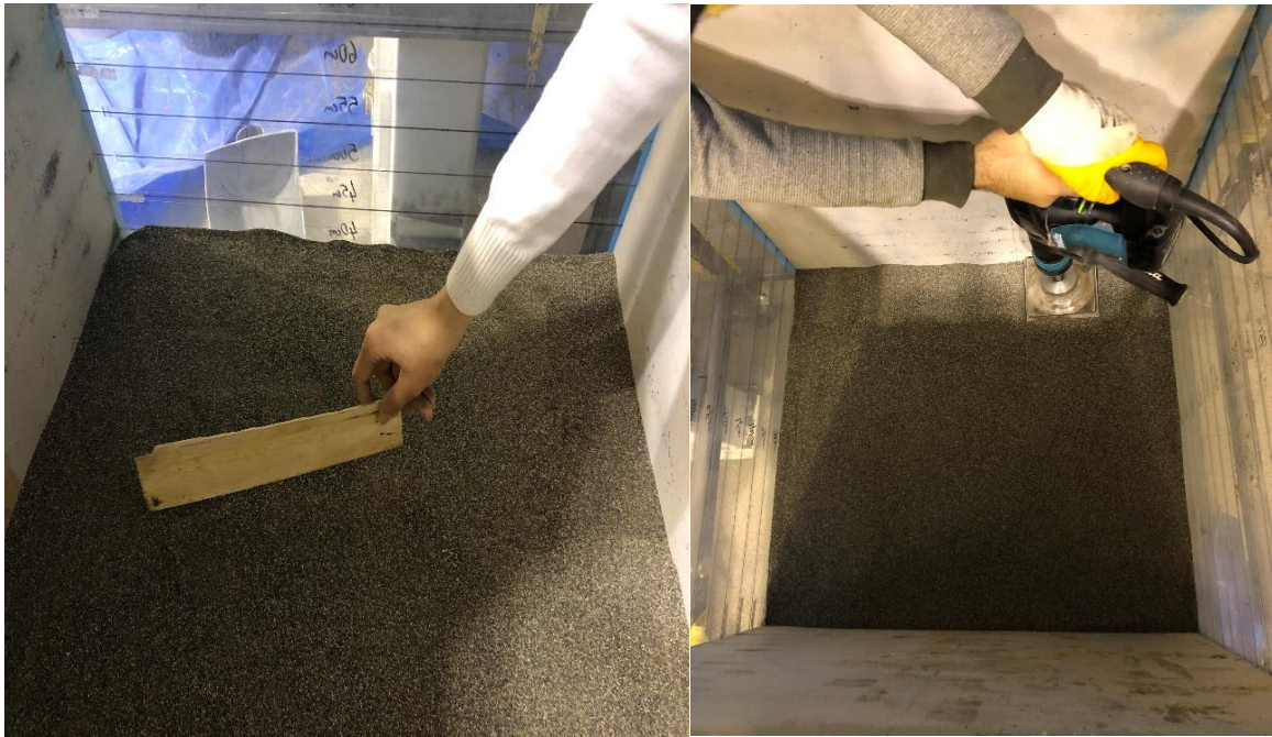
Figure 3.11. Leveling and compacting sand in the tank
