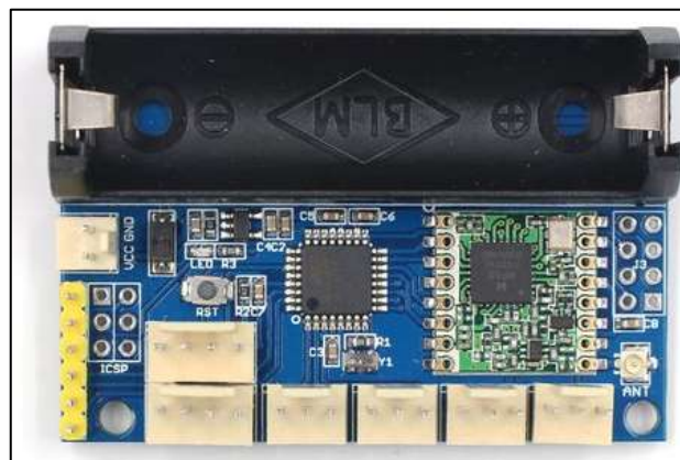
Figure 3.5: The ATmega328P LoRa Radio Node v1.0
