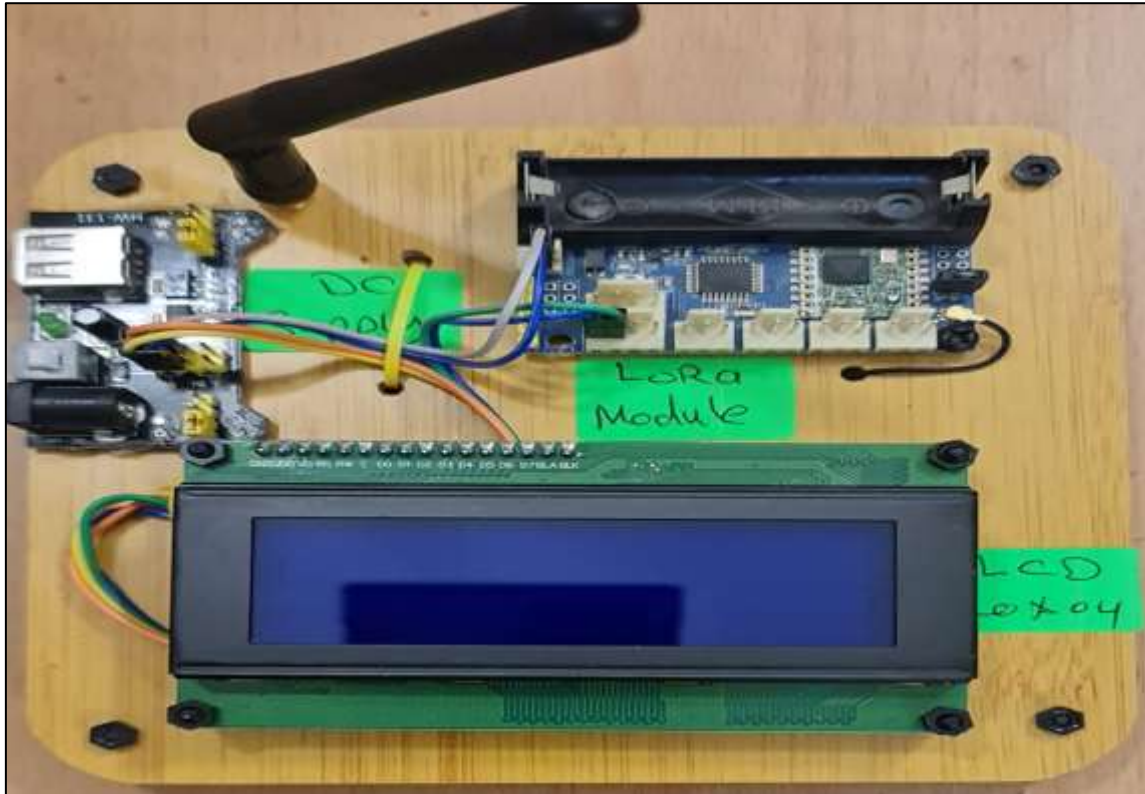
Figure 5.3: Monitoring Circuit Design for The PV System's Real-Time Performance.
