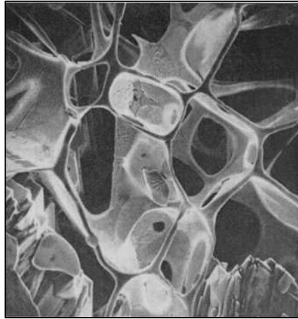
Figure 4.14. Scanning electron micrograph of sintered polycrystalline ZnO-0.5 mol% Bi 2 O 3 after the ZnO grains were dissolved in NH 4 Cl solution (x1780) [122].
