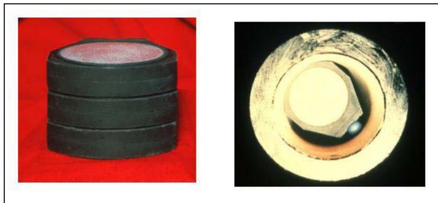
Figure 4.3. ZnO varistor components used in the construction of high voltage station arrester shown in Figure 4.2 [91].
