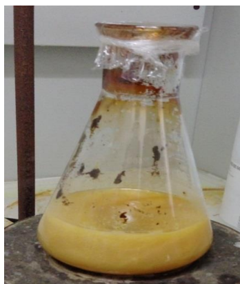
Figure 5.1. The yellow slurry of Graphite Oxide product after adding H 2 O 2 .
